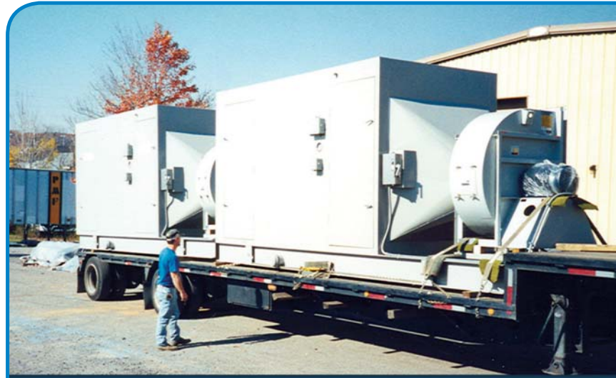
Continuous Cleaning Units
